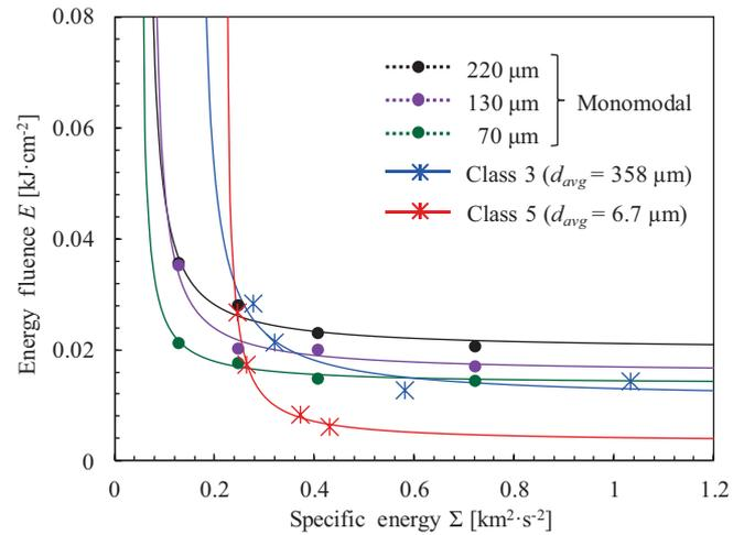
Figure 1 Computationally predicted 50% thresholds for the monomodal systems having the average grain size of 70, 130, and 220 μm and experimentally measured thresholds for pressed class 3 ( $d_{avg} = 358 \mu\text{m}$ ) and class 5 ( $d_{avg} = 6.7 \mu\text{m}$ ) HMX powders.
