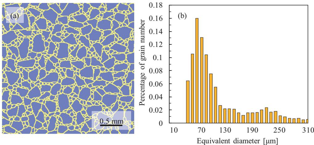
**Figure 4** (a) is the cross sectional view of the bimodal system that has the size distribution shown in (b).
