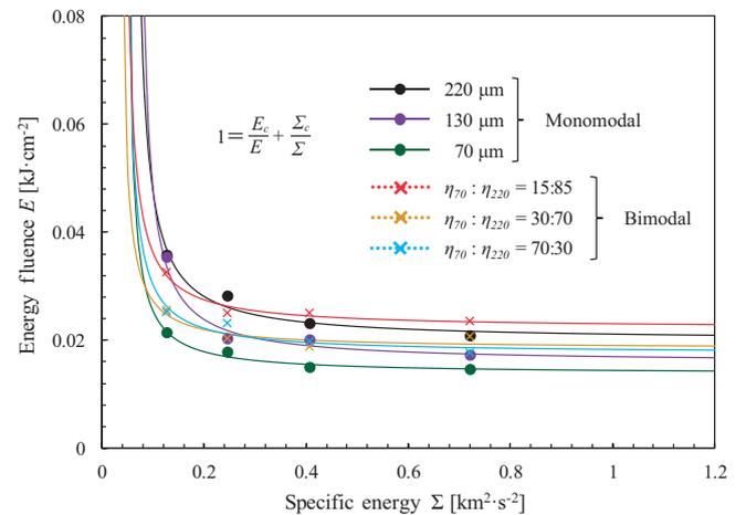
Figure 2 Predicted 50% ignition thresholds for the bimodal systems in comparison with the base monomodal systems<sup>7</sup>. Solid and broken lines are James functions fitted to discrete computational points.
