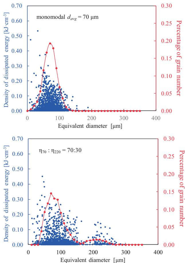
**Figure 5** Comparison of the calculated dissipated energy and the particle size distribution as a function of equivalent diameter for the monomodal system having  $d_{avg}$  of 70 μm and the bimodal system consisting of  $\eta_{70} : \eta_{220} = 70:30$ .
